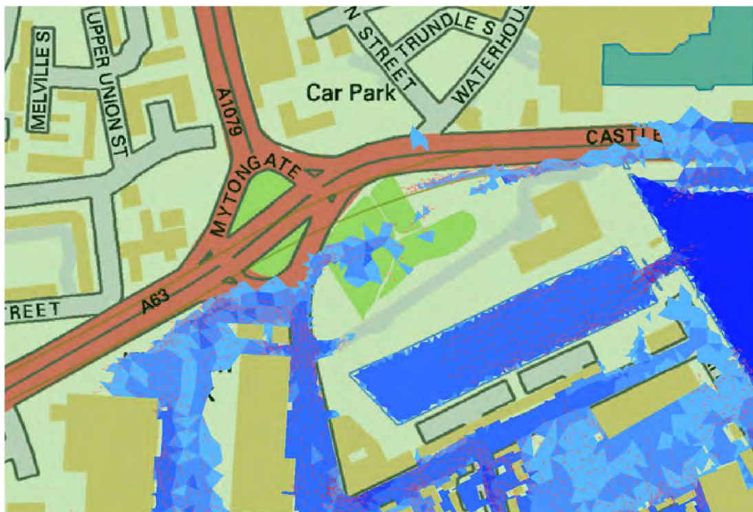
Figure 10-1 – Flow propagation for a 1 in 200-year Humber wave overtopping event at simulation time 12hrs 12mins
